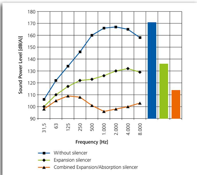
The acoustic design covers two main steps: the determination of the non-silenced sound power level and calculation of the silencer itself.
